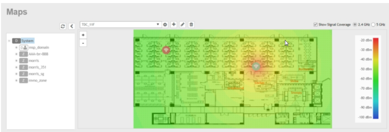
FIGURE 32 RF Coverage Heat Map
